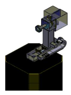
The motors can be operated separately by means of the manual control system and move along special acceleration and decellaration ramps designed to restrict vibrations. They can be manoevered independently or simultaneously with a touch-pad manual control system, equipped with emergency switch, or directly from the computer.
