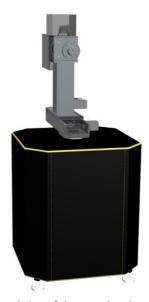
The angular resolution of the encoders is equal to 4/100° (13 bit) and the angular positions are shown on screen during measurement along with indication of the state of progress of measurement and the polar diagram of the plane under examination.
